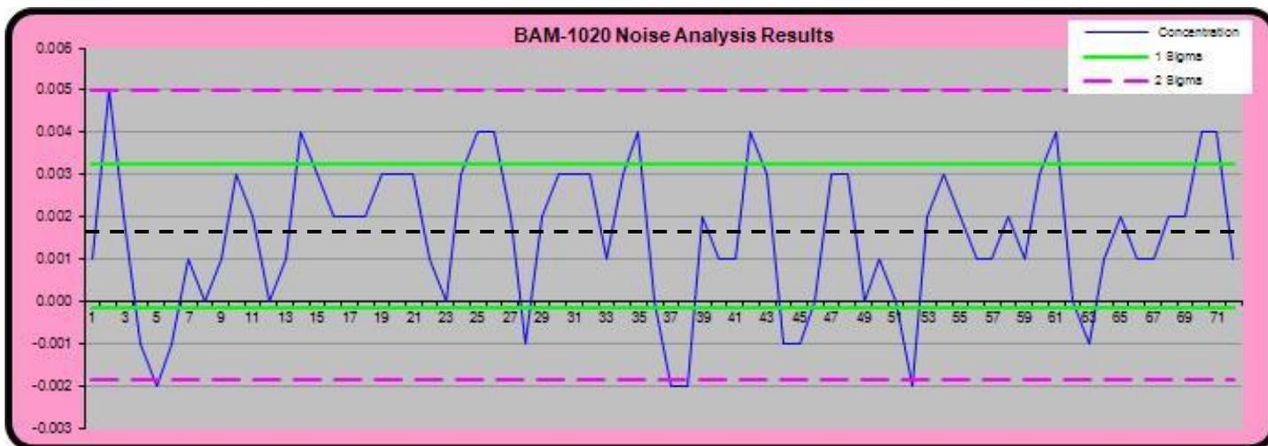
**BAM-1020 Zero Test Analysis With 1.6µg Average, 1.7µg Hourly Standard Deviation, 3.4µg Hourly Detection Limit**
