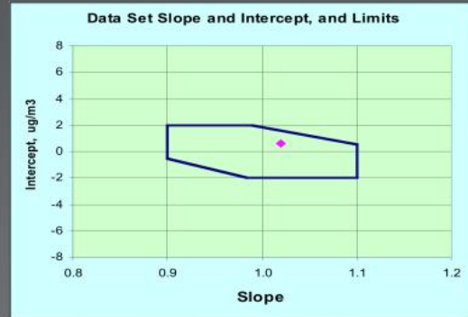
Linear regression and acceptance window of an improved PM2.5 FEM BAM-1020 compared to FRM, showing good results.
